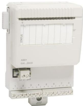
The AI801 Analog Input Module has 8 channels for current input. The current input is able to handle a short circuit to the transmitter supply at least 30 V d.c without damage.
